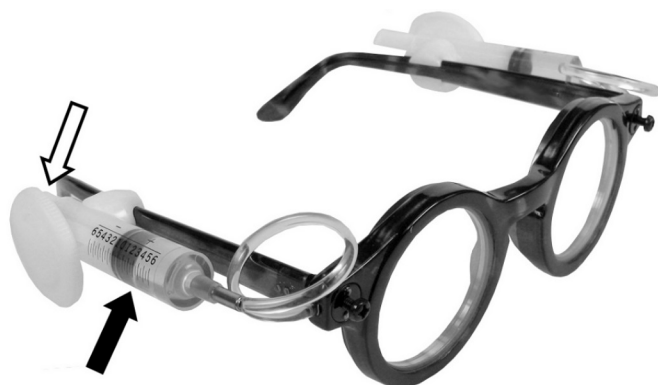
Fig 1 Adjustable spectacles: open arrow indicates adjustment knob, solid arrow indicates diopetre scale on user controlled pump. Lens can be sealed and adjustment mechanism removed after desired power is obtained
